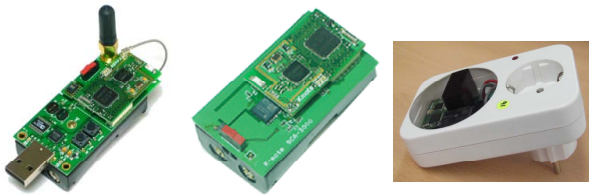
Figure 3. Diverse Wireless Sensors (temperature, humidity, acceleration, electric power meter)
